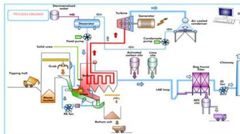
of EfW plant will be configured using simple non-reheat Rankine Cycle concept with
