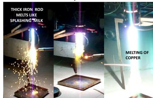
Figure 4 .The plasma jet from air plasma Torch (Developed in BARC)
