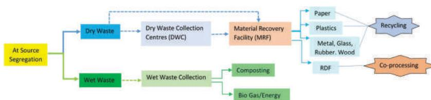
The stages in MSW waste management: Several DWC can be set up with MRF or waste can directly reach MRF. At higher scale, the role of MRF, with automation and technology, becomes important for a sustained demand and supply chain management. On the other hand for wet waste, several other technologies can be taken up.
