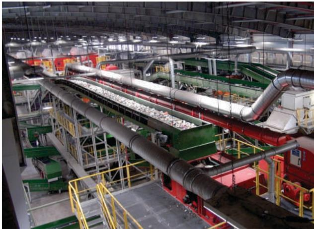
This unique plant in Hiriya enables the extraction of alternative fuel from solid waste, which serves as an energy source for the Neshet cement factory. It is a groundbreaking project, the largest waste management project undertaken so far in Israel.
