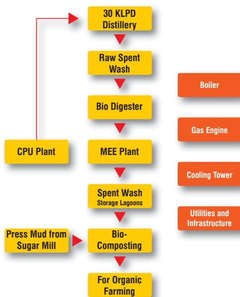
**Material Balance for Zero Liquid Discharge (ZLD) Scheme through Bio-composting for a typical 30 KLPD Distillery**
