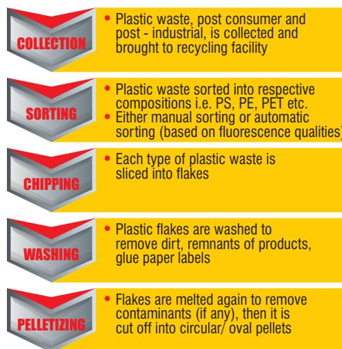
Figure 1 Mechanical Recycling of Plastic Waste (Adapted from QDB, 2017)
