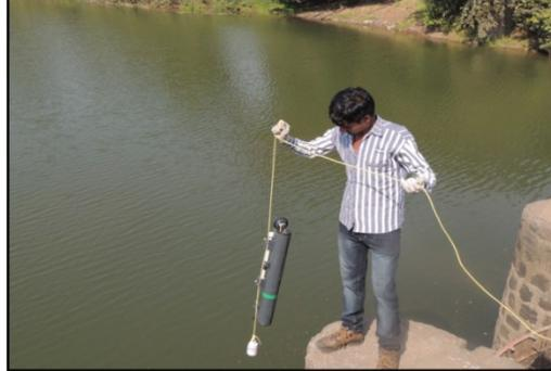
**Collection of phytoplankton sample using Niskin sampler In Indrayani River**
