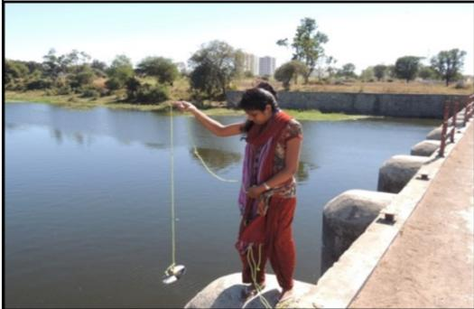
**Secchi disc being operated for transparency measurement at Wakad bandhara**
