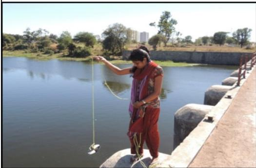
**Secchi disc being operated for transparency measurement at Wakad bandhara**
