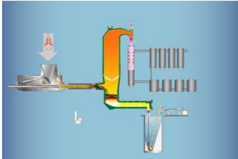
**Figure 6:** The Thermoselect gasification process.<sup>19</sup>
