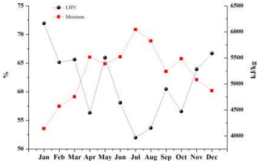
**Figure 3:** Moisture content and heating value of Shenzhen city at 2011.<sup>15</sup>
