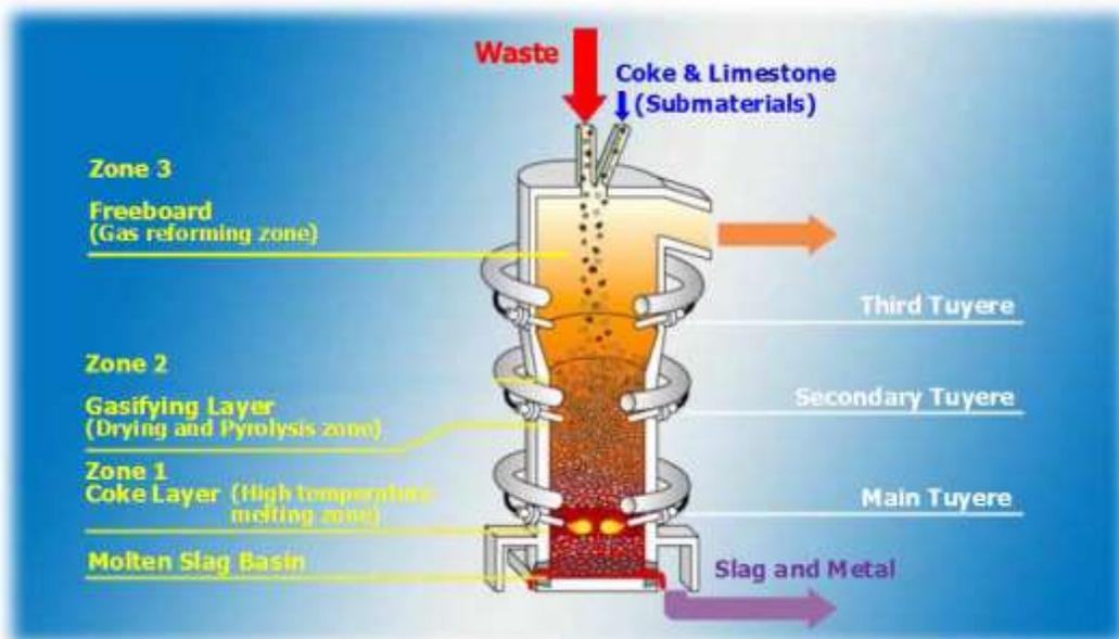
Figure 4: The JFE Direct Smelting process.<sup>17</sup>
