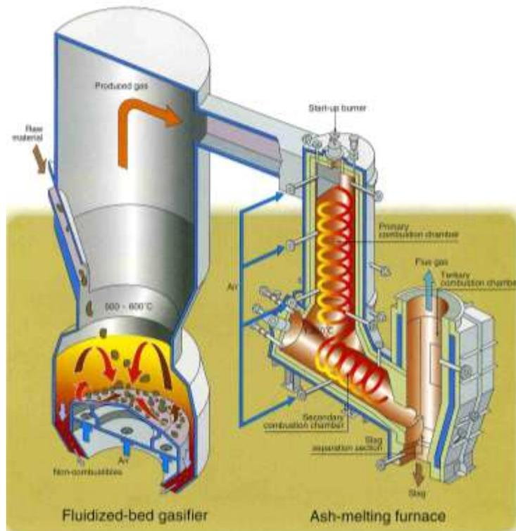
Figure 5: The Ebara fluid bed gasification process.<sup>18</sup>
